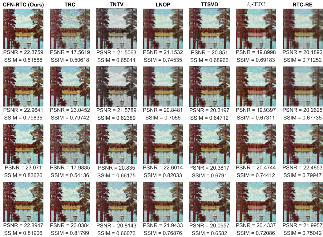
Fig. 5. Recovered Scenery images by different algorithms. The first and second rows contain the results with the random mask with impulsive noise and Gaussian noise, respectively. The third row shows the restored images with the deterministic mask and impulsive noise, while the fourth row contains the reconstructed pictures with deterministic mask and Gaussian noise.
